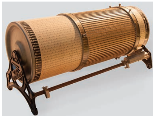
Figure 4. The world's largest and most precise mass-produced logarithmic cylindrical slide rule Loga calculator. Scale length: 24 m (courtesy of Konzernarchiv UBS).
